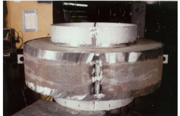
Lining (inner cylinder) of exhaust ducting in pulp and paper recovery boiler made from HR-160® alloy. Outer shell is carbon steel.
