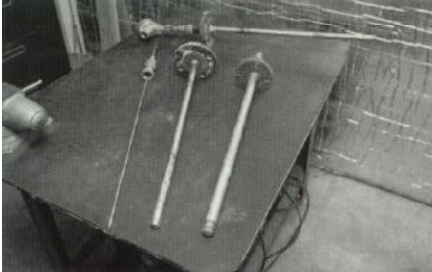
Many waste incineration and chemical process facilities have used HR-160® thermocouple protection tubes with outstanding success. Life extensions greater than 10X compared to Ni-Cr alloys and stainless steels are common.
