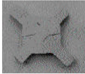
STELLITE 6 Hot cracked at 3rd layer (stopped after 24 beads)
